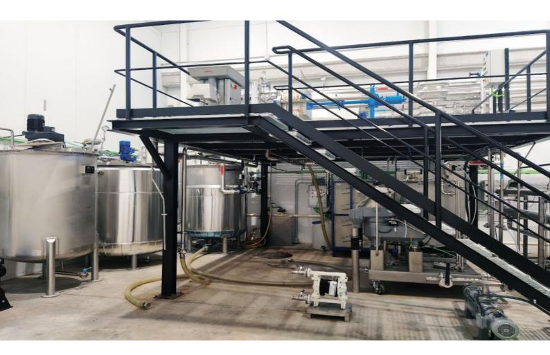
The SAV bioprocess demonstration plant (TLR6-7) provides a biotechnology laboratory and a pilot plant with the necessary equipment (stirred reactors, bioreactor, filtration and centrifugal units, distillation units...) for the development of various types of bioprocesses, having experience in the framework of the circular economy.
