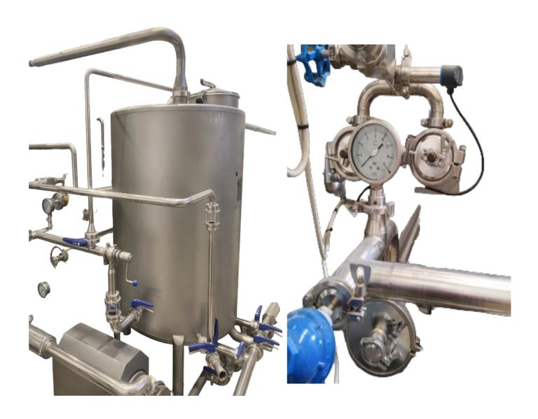
Total volume of 1.5 m<sup>3</sup>, capacity 500 l/h, ultrafiltration 10 kDa, nanofiltration 200 Da.
